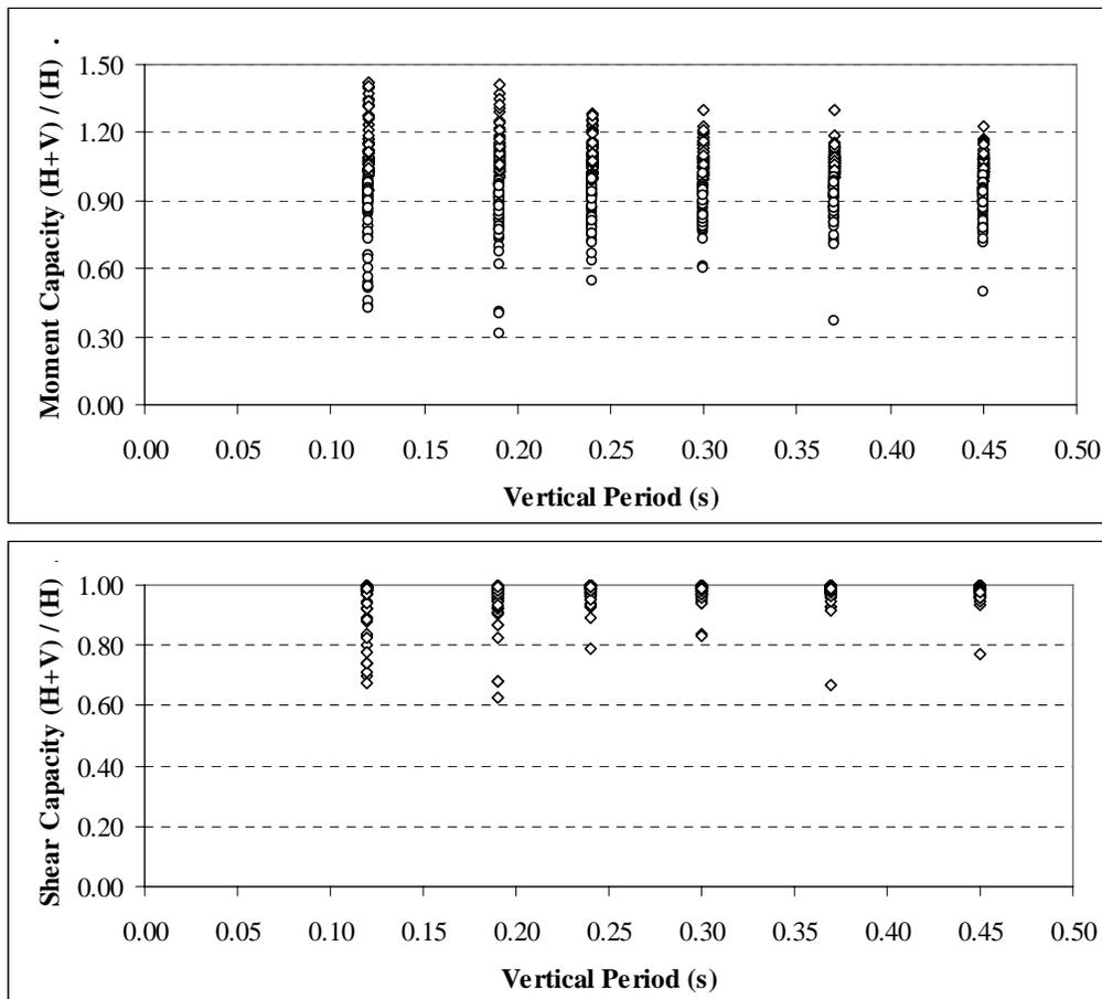
Figure 6 – Variation of column moment and shear capacity due to vertical effects
