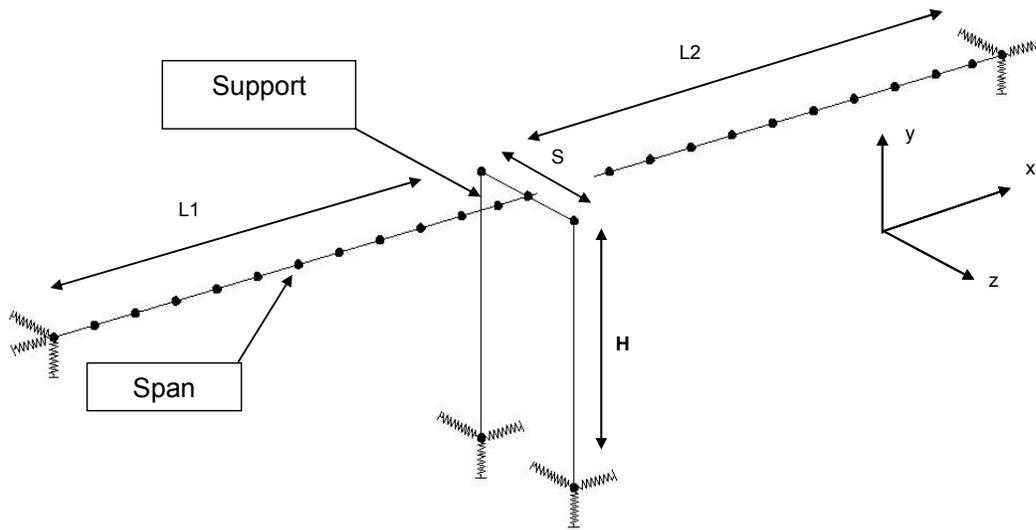
Figure 2 – Simulation model of the Camino Del Norte bridge
