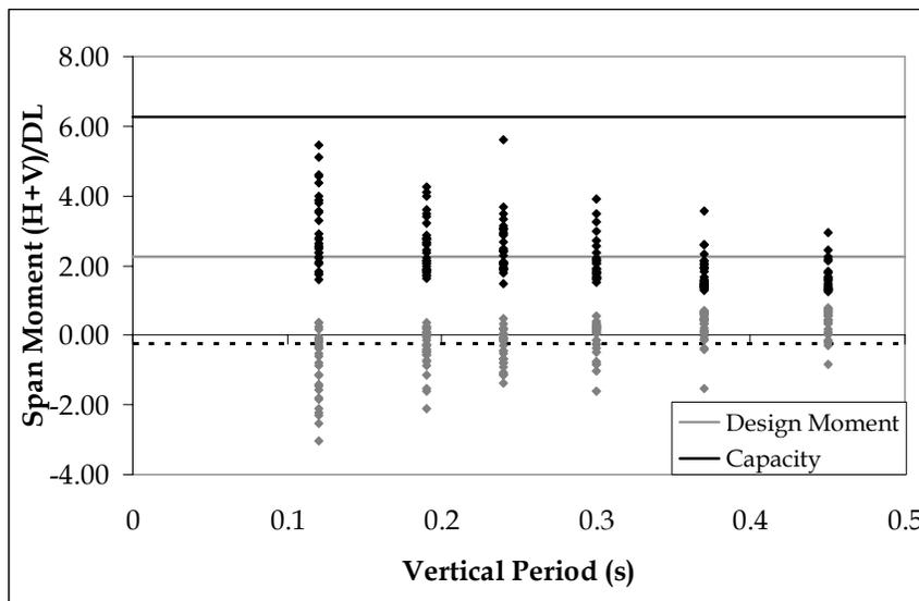
Figure 5 - Variation of moment demand at the mid-span with vertical period for unscaled ground motions
