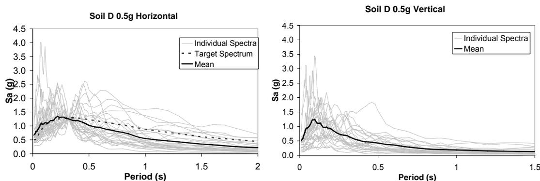
Figure 3 –Spectra of the horizontal component of ground motions scaled to match the ARS curve (Magnitude 8.0, PGA 0.5 g and site class D) at fundamental longitudinal period of base configuration, and corresponding vertical spectra
