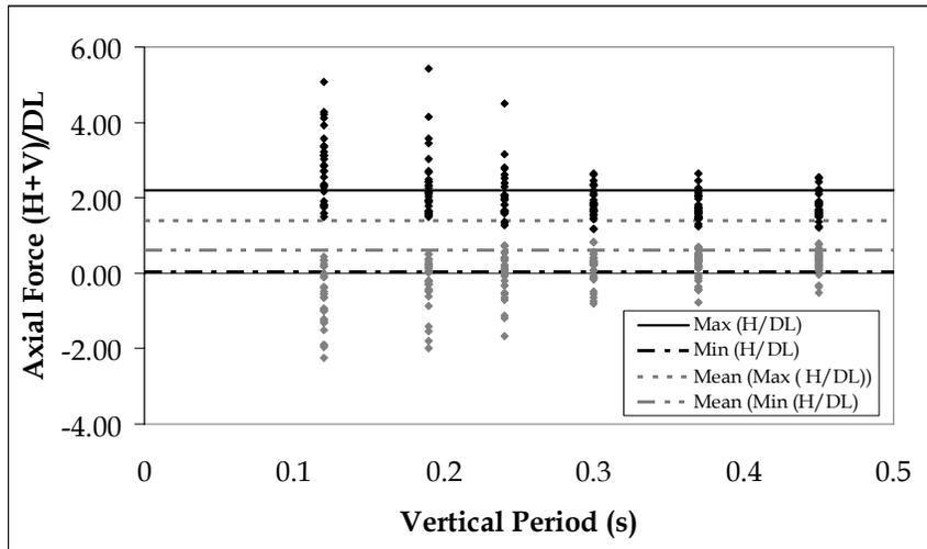
Figure 4 – Variation of column axial force demands with vertical period for unscaled ground motions
