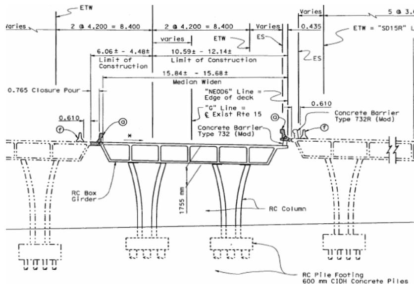
Figure 1 – Elevation view of the new segment of the Camino Del Norte Bridge
